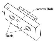
**Caution:** Do not touch the reels during loading and unloading. It could cause injury or damage the cassette adapter or tape.
